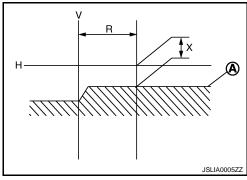
5. Adjust the cutoff line height (X) with the aiming adjustment screw so as to enter in the adjustment range (M–N) according to the horizontal center line of headlamp (H).
